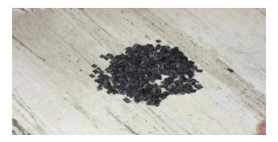
Figure 1: Rubber Tyre Chips
