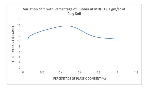
Figure: 3 - Variation of  $\phi$  with Percentage of Rubber at MDD 1.67 gm/cc of Clay Soil
